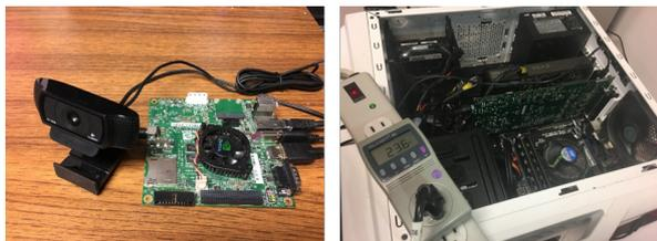
Fig. 5: Left: Front-end (Tegra TK1 and webcam); Right: Back-end (Xilinx VC709 FPGA board, host PC)
